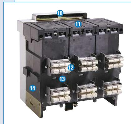
This rear view of a Magnum drawout breaker shows the designed-in safety feature of locating the primary disconnects and secondary contacts on the removable breaker element for easy and safe inspection.
