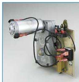
An electric motor automatically charges the closing springs. In absence of control power, the springs can be manually charged.
