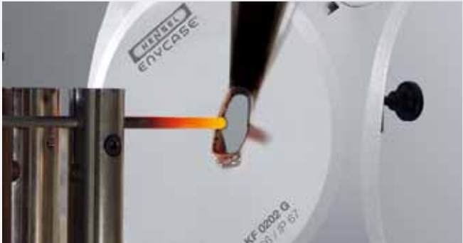
Burning behaviour in glow wire test 960°C High impact withstand IK 09 (10 joule)
